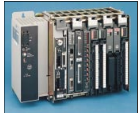
Figure 2. PLCs typically use vendor-specific communications protocols that require specialized hardware interfaces and software drivers.
